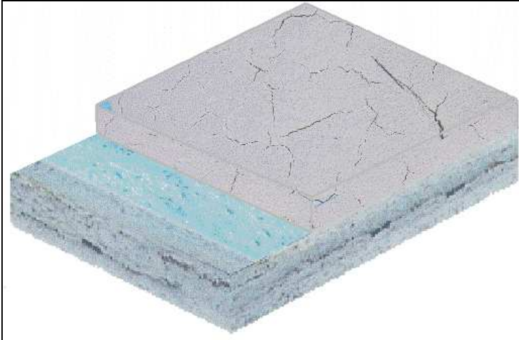
Figure 1. Water-base polyamine adduct epoxy shrinkage cracking.
