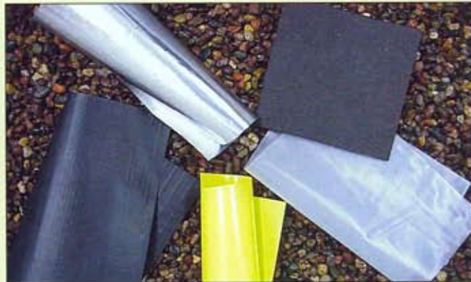
Many types of vapour retarder sheet materials are available. In recent years, puncture and tear-resistant materials with extremely low permeability have become available and are preferable over ordinary polyethylene sheet. Vapour retarders should be specified to meet the requirements of ASTM E 1745, Standard Specification for Plastic Water Vapour Retarders used in Contact with Soil or Granular Fill under Concrete Slabs.
